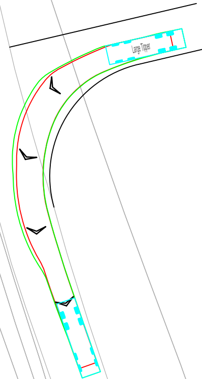
Tipper Vehicle Exiting Site
